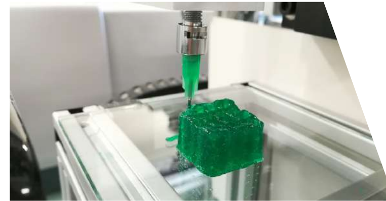
Image: stable complex 3D structure obtained through the 3D printing of cross-linked alginate using a new in situ process
