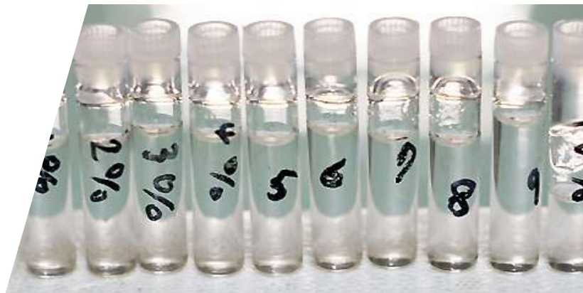
Gelling of a cellulose solution dissolved in LiCl/DMAc by adding increasing volumes of water
